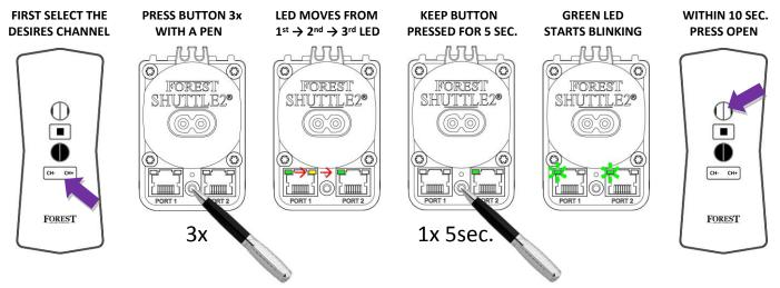
When after several attempts the motor doesn't react to an open or close comment, you might have reset the end limits by accident. Try to set the end limits again.
