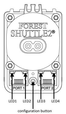
Use a pin to change settings in the configuration menu. Choose the setting you want to change (table below) and press the button that many times (corresponding with setting).
