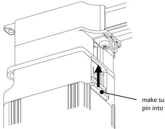
make sure to secure the locking pin into the motor pulley
